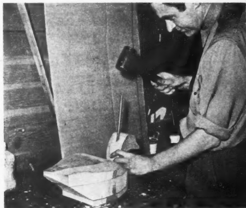
Bore a \frac{3}{8} -in. hole through head into body (at an angle to prevent head twisting on its axis), fit a dowel in the hole, and glue head in position.
